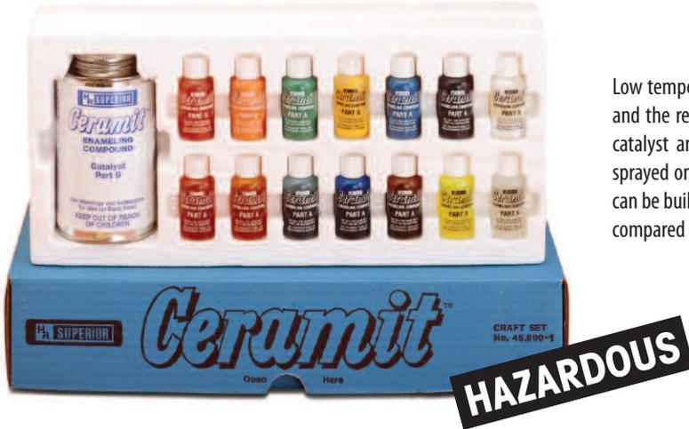
Low temperature curing, hard enamel. Requires only 200° F (93° C) for one hour and the result is a ceramic-like surface. A two-part, liquid system, in which the catalyst and the color are mixed in a 2-to-1 proportion. Can be brushed on, sprayed on or applied with a spatula or squeeze bottle. Apply in a single coat or can be built up in successive layers. Has a hardness of 60-75 on the Sward scale, as compared to kiln-fired enamel 65-80, which requires 1500° F (816° C) to cure.
