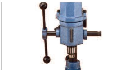
Depth gauge indicates the exact depth of the spindle in the timber. Required depth can be fixed by the stopper on the handle spindle.
