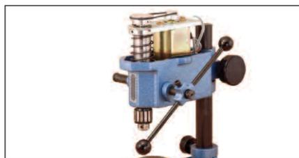
Four spindle speeds are available by belting on different pulleys.
